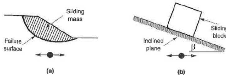
**Figure 6: Sliding Block Slope Stability Analogy**
