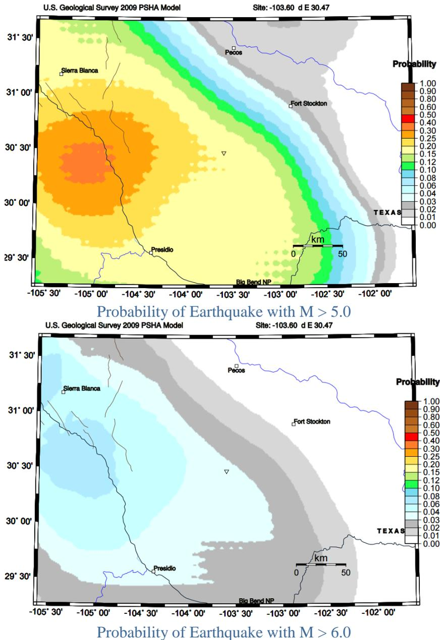
Figure 2: Earthquake Magnitude Probability – Near Center of Pipeline Alignment
