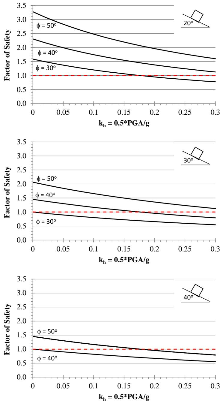
**Figure 7: Variation in Pseudostatic FS for Newmark Sliding Block Analogy**
