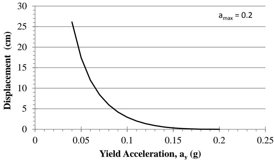
**Figure 8: Seismic-Induced Permanent Slope Displacement**
