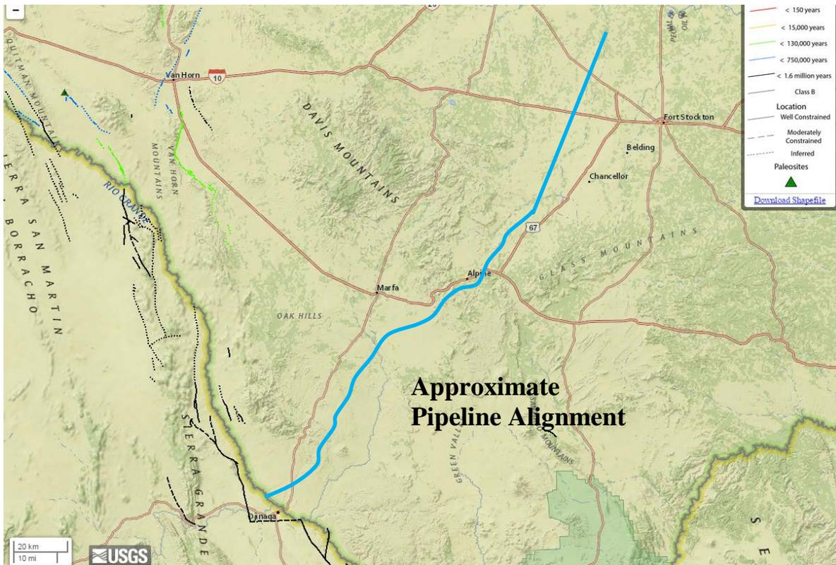
Figure 5: Quaternary Faults near Pipeline
